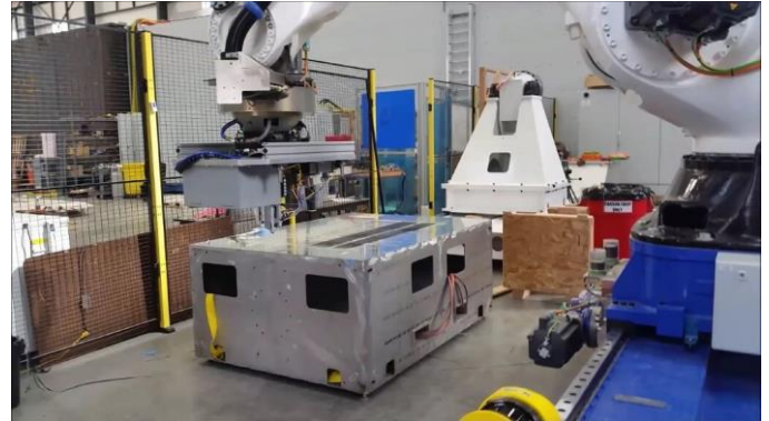
Figure 10 - Robot prototype laying up material on tape
